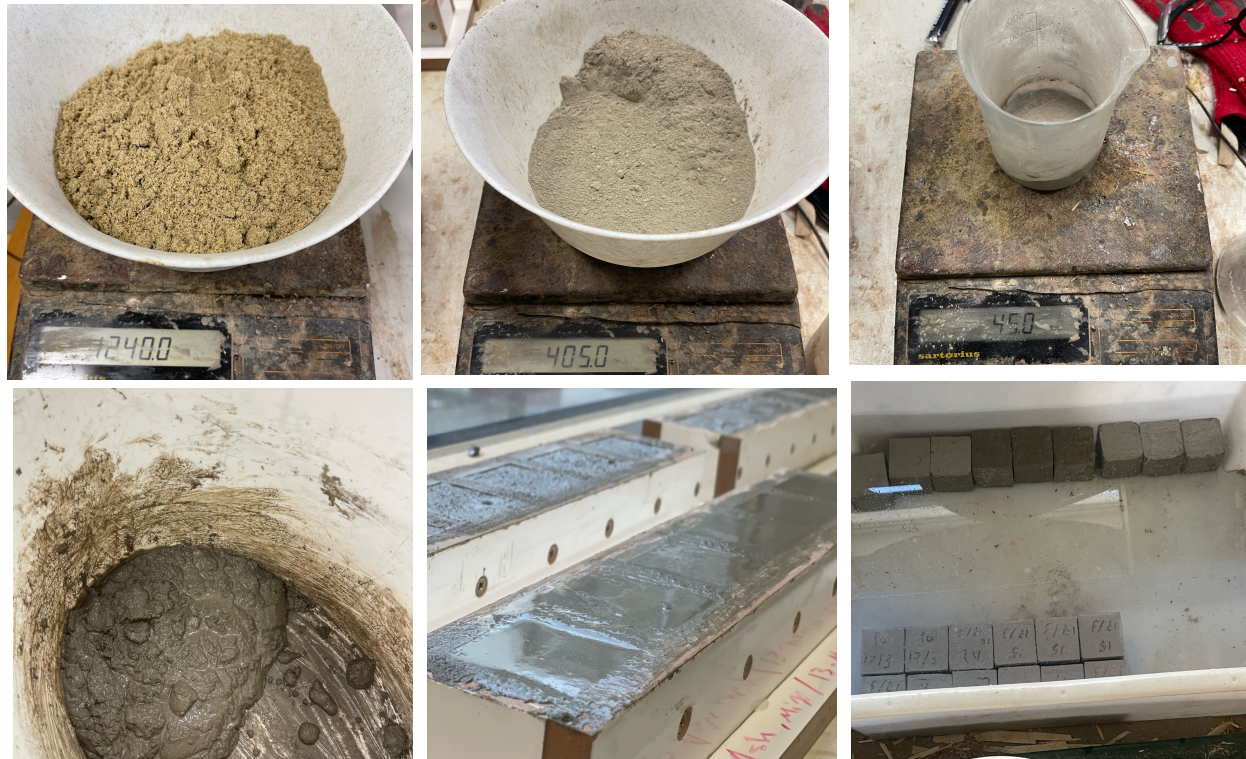
Figure 9: Laboratory Procedure for Mixing, Casting, and Curing of Mortar Specimens with Partial Cement Replacement Using Ash.
