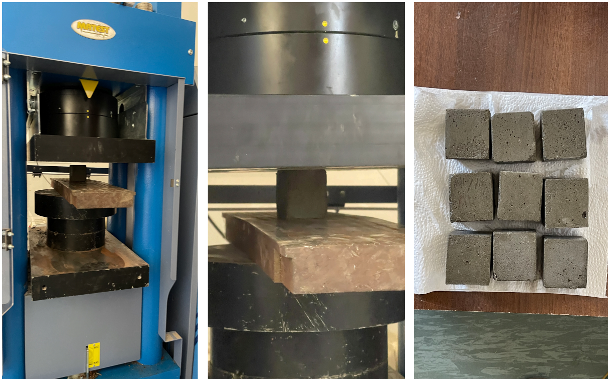
Figure 10: Compressive Strength Testing of Mortar Cubes Using a Servo-Controlled Hydraulic Press in Accordance with ASTM C109.
