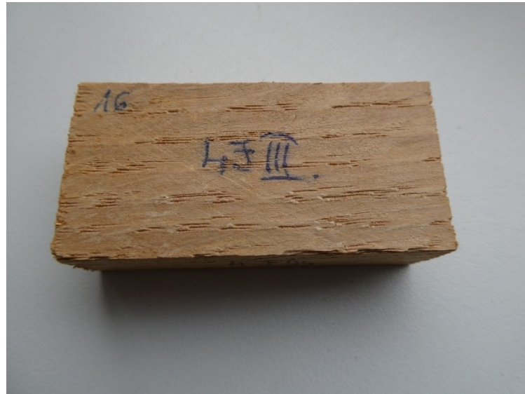
34. ábra: a labirintus tapló bontotta 4JIII- as minta
